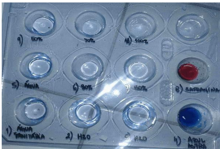
Figure 1 – Sequence of the staining procedure for plant material sections. (1) Hypochlorite; (2, 3 and 5) Water; (4) Astra blue dye; (6) 30% alcohol; (7) 50% alcohol; (8) Safranin dye; (9) 50% alcohol; (10) 70% alcohol and (11) 100% alcohol
